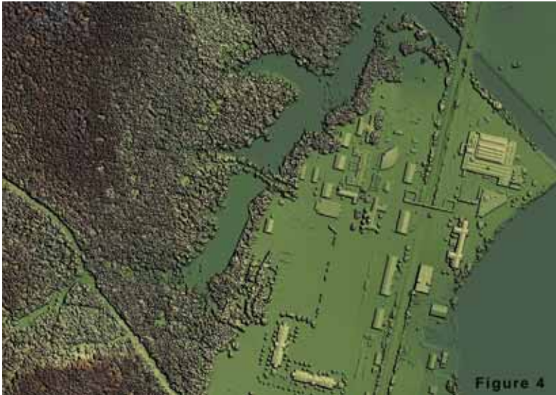
Fig 4: Color shaded relief intensity map of portion of Chopawamsic Creek map, Quantico Marine Base, Quantico VA. Note ability to see single buildings, trees and even vehicles.
